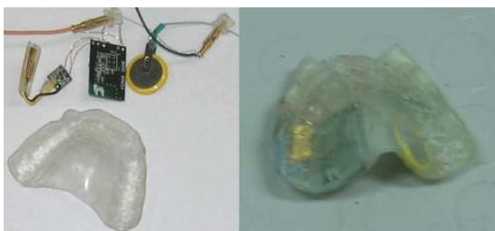
Fig.4. Instrumented splint before and after of assembly process
