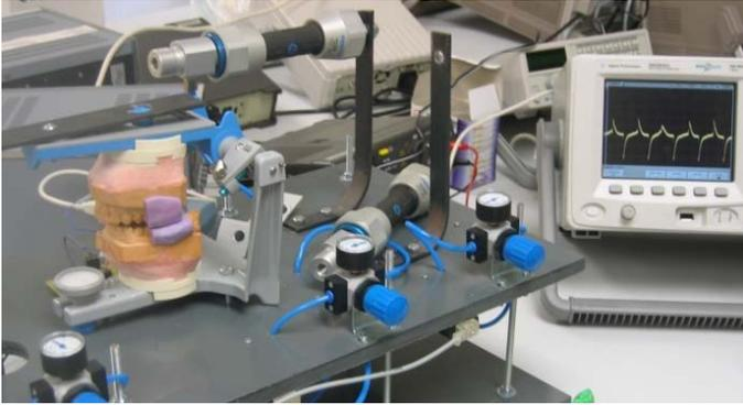
Fig. 3. First trials: The oscilloscope shows sensor output voltage on applying levels of pressure as input.
