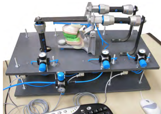
Figure 9: Bruxism simulator with pneumatic operation for the “in vitro” trials.
