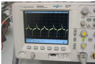
Figure 7: First trials: The oscilloscope shows sensor output voltage on applying levels of pressure as input.
