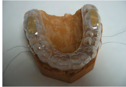
Figure 8: Splint with piezoelectric sensors for diagnosing bruxism.
