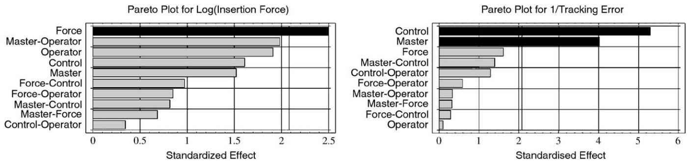
Fig 8. Left: Pareto plot for log (insertion force). Right: Pareto plot for 1/tracking error. Black bars means significant factors.
