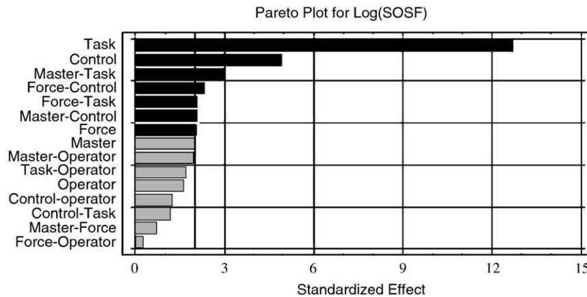
Fig 6. Pareto plot for log (SOSF). Black bars means significant factors.
