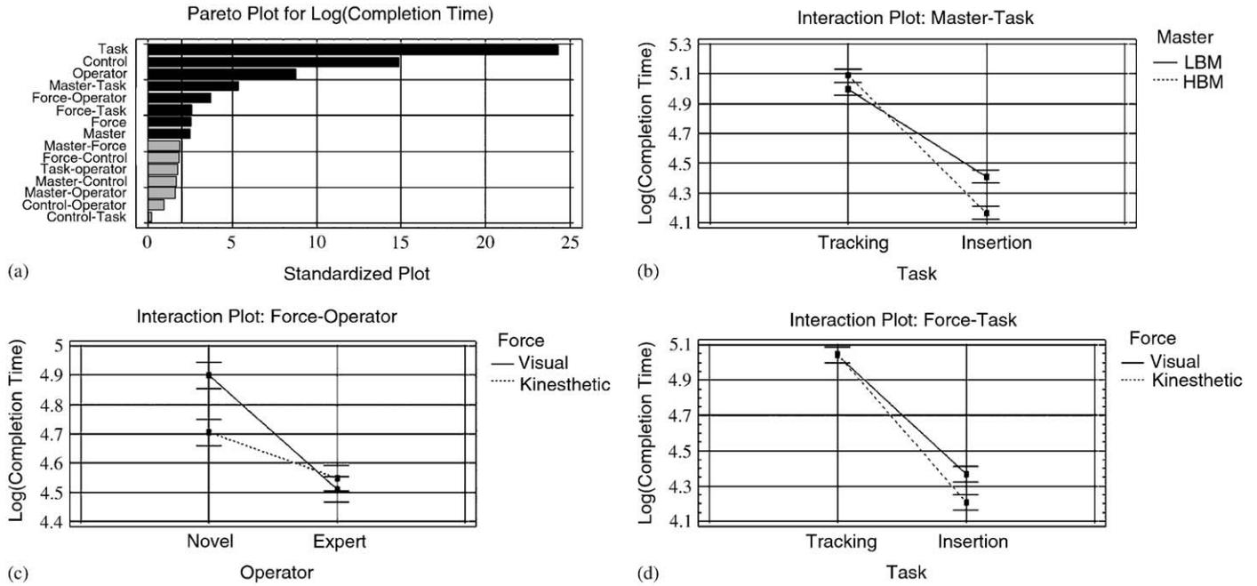
Fig 5. (a) Pareto plot for log (completion time). Black bars means significant factor. Significant interactions for log (completion time) (s). (b) master–task. (c) force–operator. (d) force–task. (95% LSD interval).
