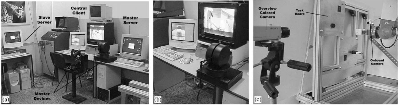
Fig 2. Telerobotic system PLATERO: (a) devices overview; (b) man–machine interface; and (c) remote zone.
